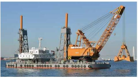
GE Series (All Electric Crane with Hybrid System)
