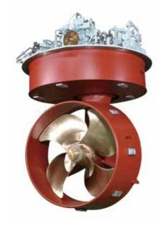
Recently built LNG-fuelled tugboats are KST Liberty and Maju Loyalty operated in Singapore, owned by Keppel Smit Towage/Maju Maritime, a joint venture of Keppel and Royal Boskalis Westminster. Each is equipped with two 6L28AHX-DF main engines each of 1,920kW, and two NIIGATA ZP-41 fixed pitch azimuth thrusters.
